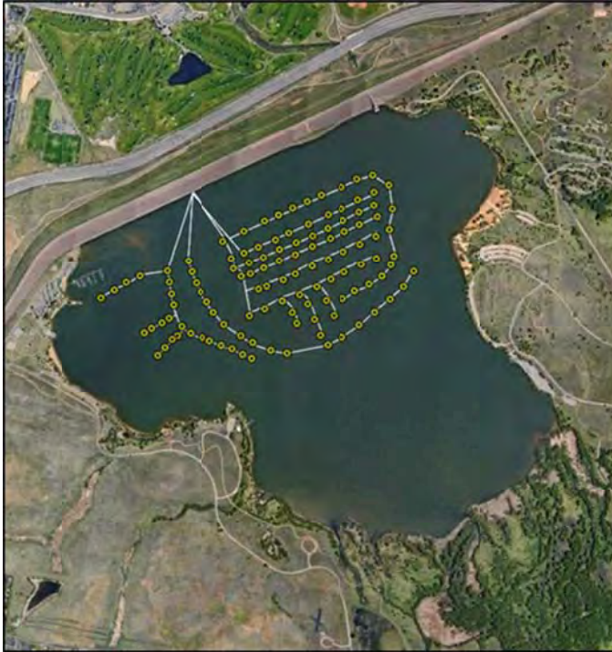
Figure 1. Cherry Creek Reservoir and Destratification System Footprint ( Background aerial image from Google Earth; imagery date May 13, 2017 )
