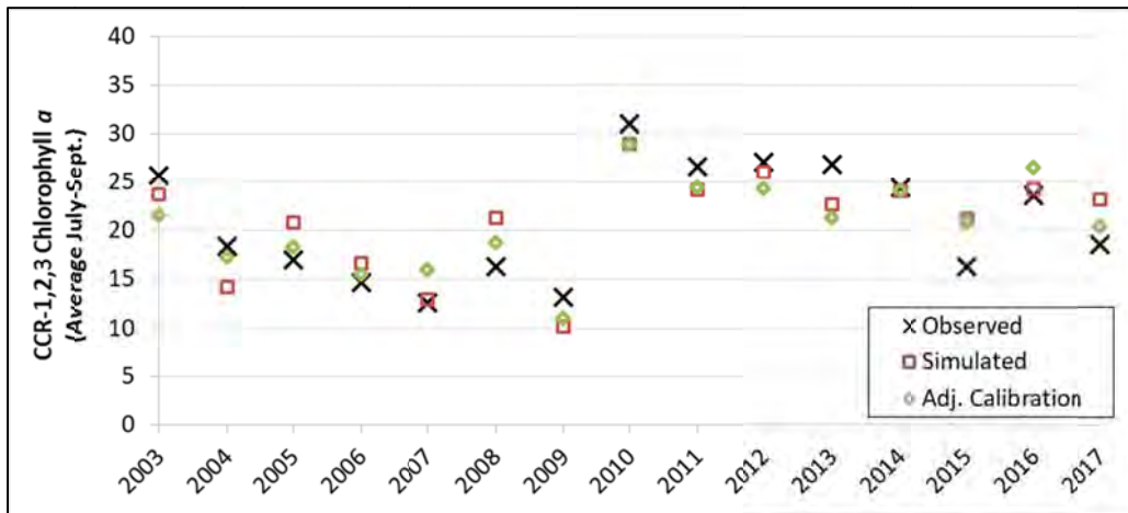
Figure ES-2. Simulated and Observed Summertime Average Chlorophyll a for Unadjusted Simulation and Proposed Calibration Refinement Run, µg/L, 2003 - 2017
